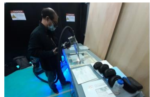
Laser Paint removal at HAECO
